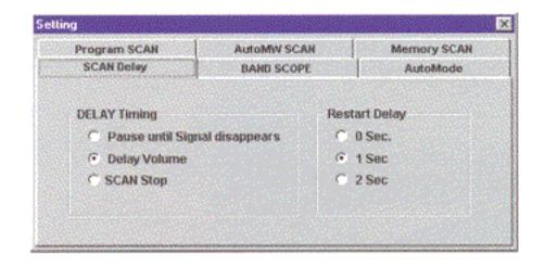
This screen allows you to select settings for various functions such as scans, band scope and the auto mode function.
