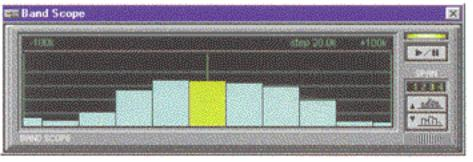
The bandscope shows signal conditions around a specified frequency.
